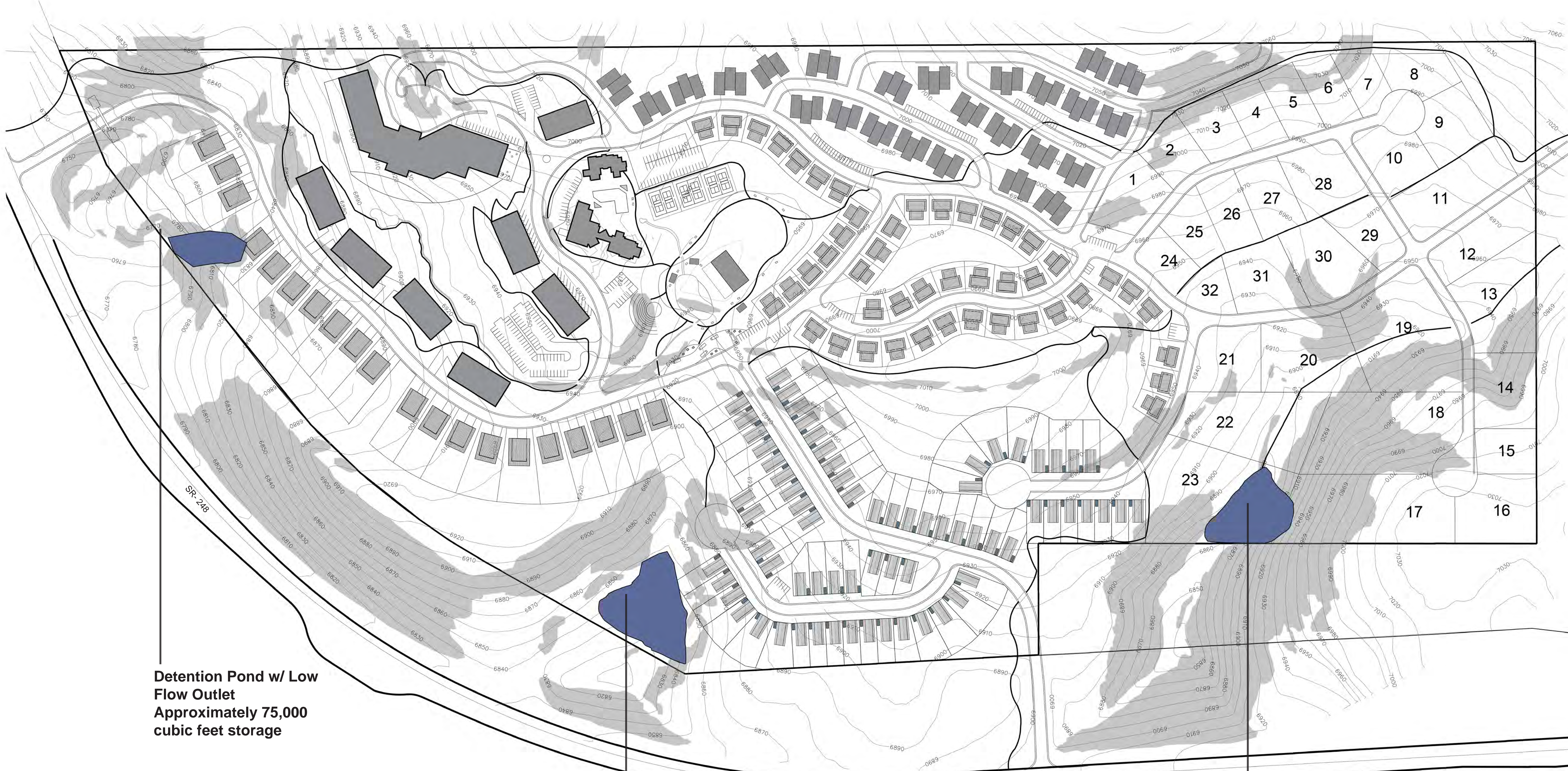
Detention Pond w/ Low Flow Outlet Approximately 90,000 cubic feet storage
